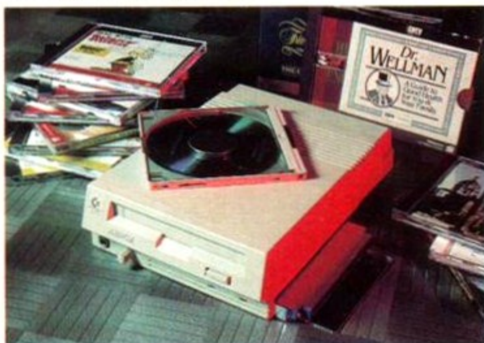
Although CD-ROM drives for different computers are incompatible, CD-ROM disks can be read by different systems. So you could use this A570 to read PC CD-ROMS. You can't run any programs, but you can look at text.
