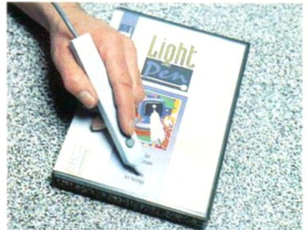
The Trojan light pen works with most programs as a mouse – but it's useless without some driver software.
